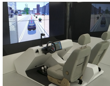
Figure 6: Autonomous Driving Simulation Platform, which is used to collect the low-level drivers’ control behavior. We learn high-level driving decisions by imitating the low-level drivers’ control commands.
